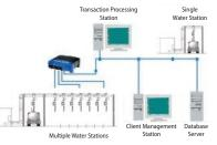
Configure one or more pipestand locations. SQL-based software runs stand alone or across a network, allowing for multi-site installations that leverage your existing TCP/IP infrastructure.
